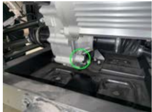
Rear gearbox oil drain plug location (Shown with rear bumper removed)
