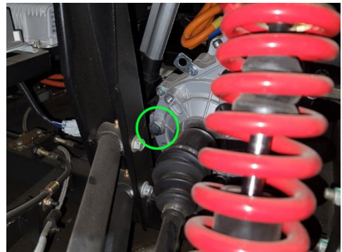
Rear gearbox oil fill plug location (Shown from rear driver side wheel well)
